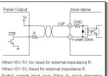
Forbid current input over 20mA to avoid damaging Photo Coupler •
